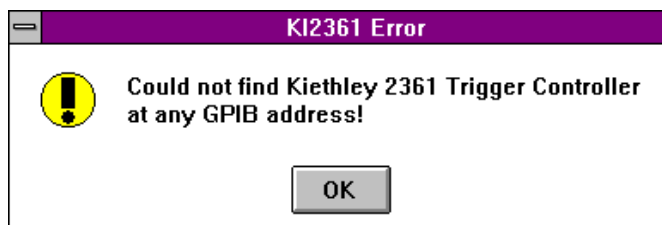
Figure 12: The Poll Function will Display an Error Message When it cannot Locate the TCU.
