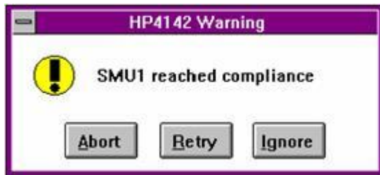
Figure 10: ICS Reports Compliance Events if the Report Compliance Switch is Selected in the Mainframe Setup Dialogue Box.
