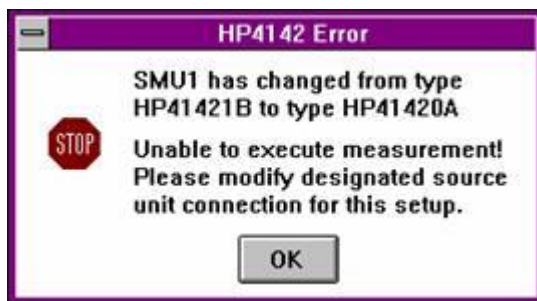
Figure 8: A hardware mismatch error is generated when either the hardware configuration stored in the project file or the hardware configuration reported by the instrument does not agree with the hardware configuration stored in memory.
