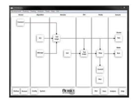
This workflow interface is separated into logical steps defining the sequence necessary to set up a device level or full wafer level test methodology. Perform system configuration and maintenance functions like backup and restore as well as launch other provided tools from the same common user interface.
